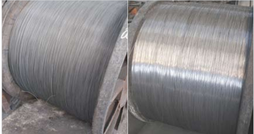
The absence of oxidation also gives the wire rod produced with the LIFE funded technologies a shinier appearance
