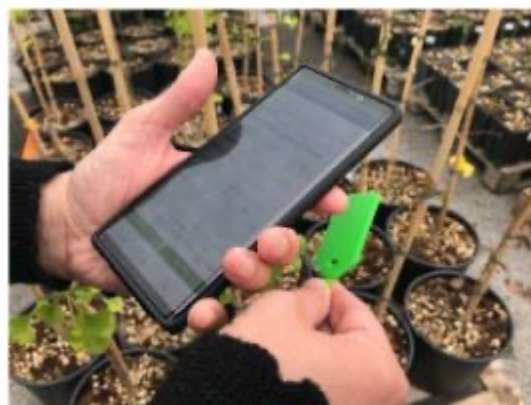
Fig. 5. Wraps NFC tag reading of the preliminary information (first section) by the app "Vivaio forestale".
