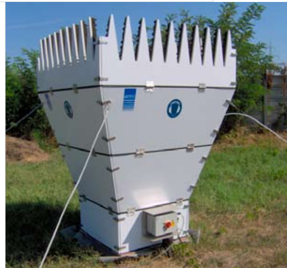
LIFE-funded monitoring equipment scans and analyses air samples from different locations providing a 3D map of real-time emissions over the city of Bucharest
