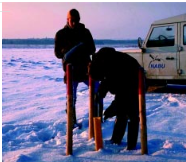
Installing gauges to monitor water levels in a fen environment. Photo © Kerstin Wernicke
