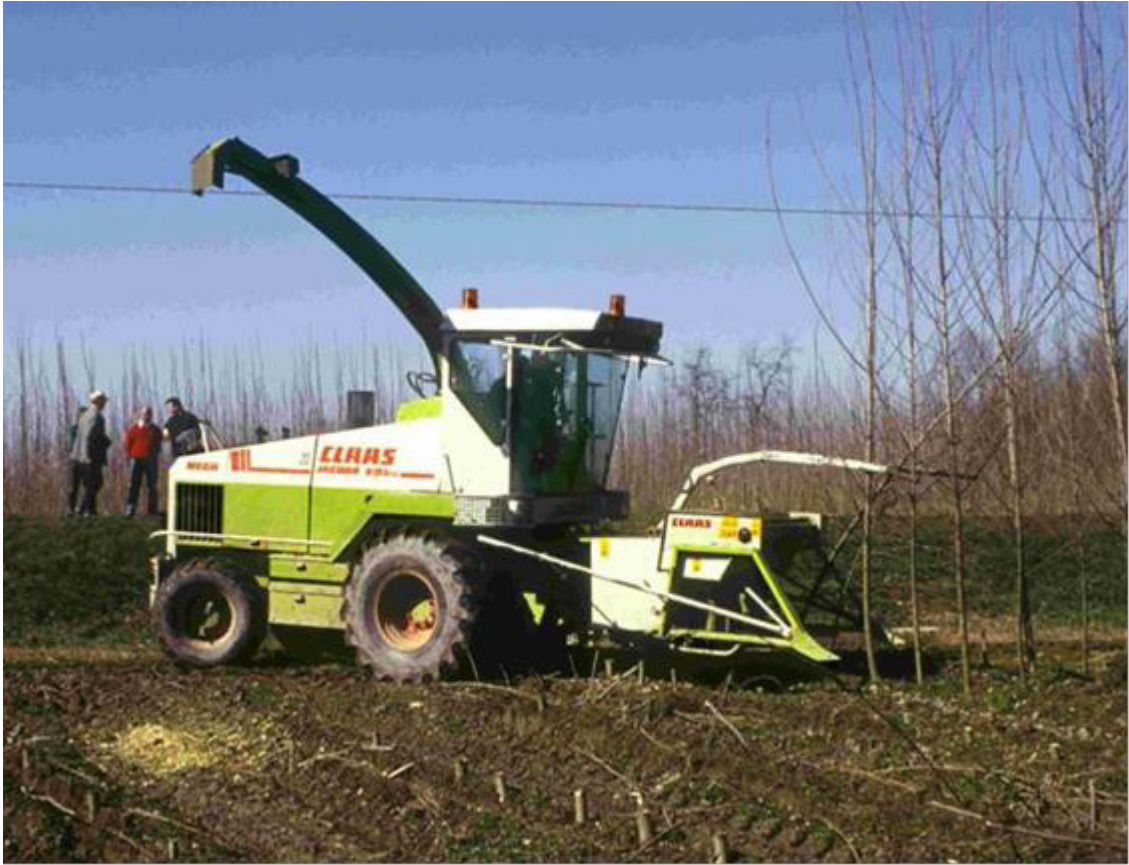
Figure 17 - Harvesting equipment for poplar biomass.
