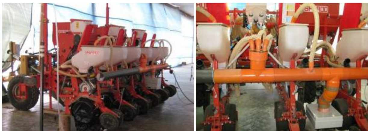
Figure 11 – Prototype 2 of CRA-ING applied to the Gaspardo Magica seeder described in point 5.3.4. The filter used in this prototype is a common activated carbon anti pollen car filter.
