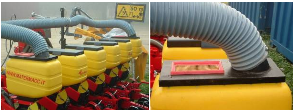
Figure 10 – Prototype 1 of CRA-ING applied to MaterMacc seeder used in APENET 2009 trials. An analogous prototype was applied to the Gaspardo MAgica seeder, adapting it to the different air deflectors. This prototype was devised as a modification which can easily be applied to existing seeders.
