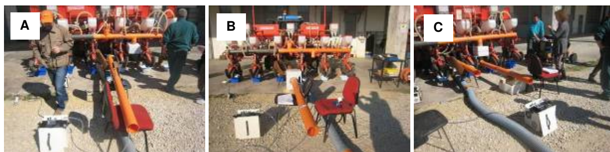
Figure 12 – A) Sampling of exiting air without filters; B) Sampling air directly editing filter; C) Sampling editing air when modification is attached to seeder ready for field use.
