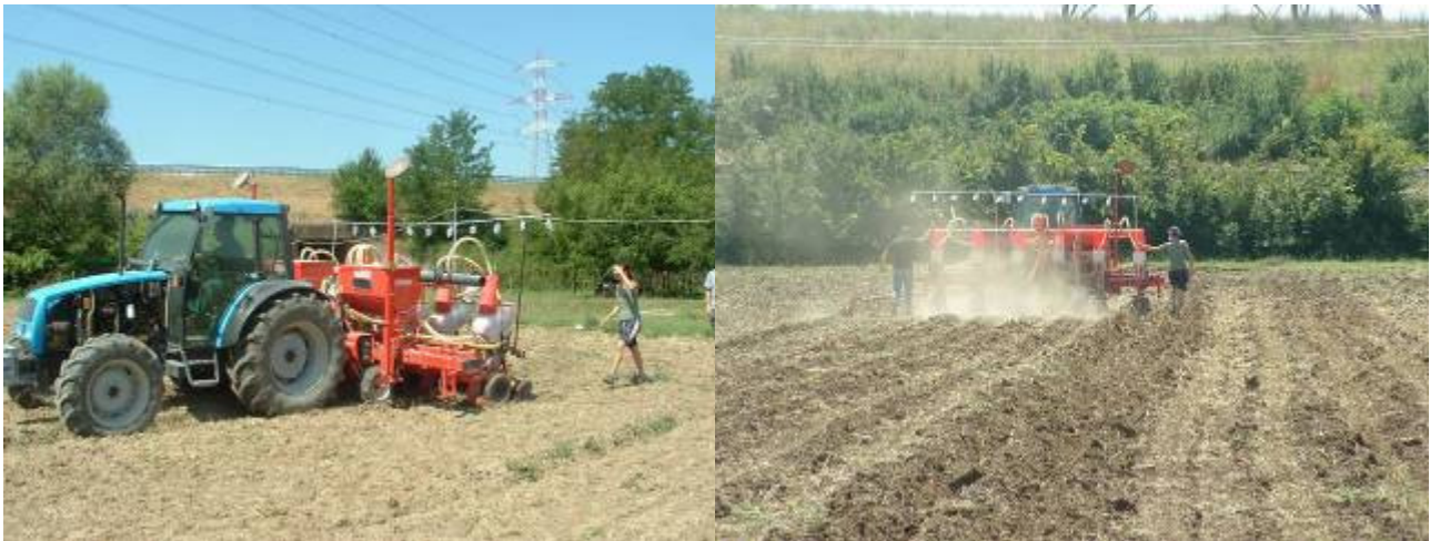
Figure 24 – Experimental group A: the horizontal bar which supports the 10 cages at 2.5 m height is fixed to the posterior part of the seeder. The picture on the right shows the system during the seeding.
