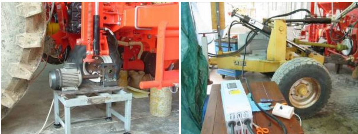
Figure 8 – Left: electric motor and inverter used to power the drive wheel; Right: electric motor and inverter used to power the depressor.
