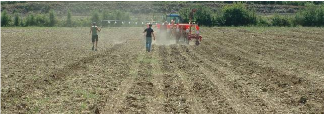
Figure 25 – Experimental group C: the bar that supports the 10 cages is kept at 1.8 m height by two operators. They proceed at 4 m from the seeder, laterally, so as to intercept the dust cloud shifted by the wind.
