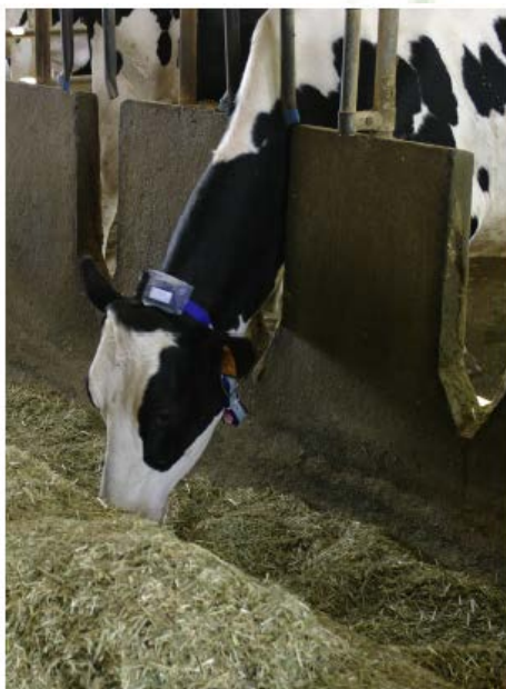
Fig. 1. SensorTag fixed to the collar of the cow.
